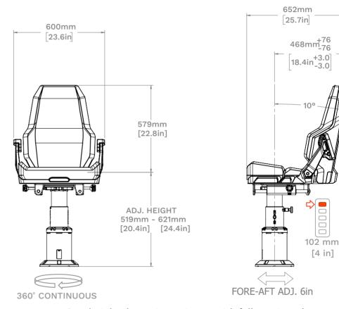
Seat height shown is maximum with fully optioned seat. Min seat height is 32.75mm lower without options.
