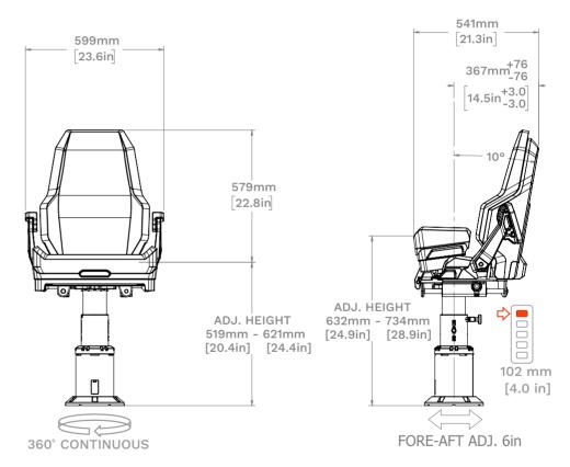
Seat height shown is maximum with fully optioned seat. Min seat height is 32.75mm lower without options.
