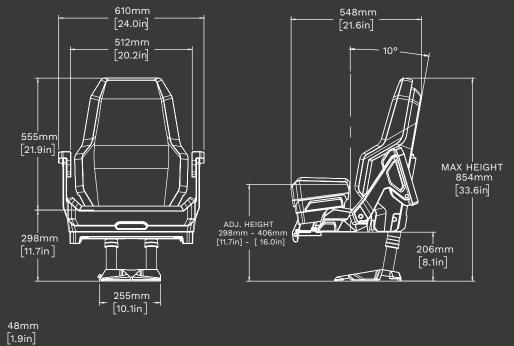
9 mm / 3.5 in 3.7 kg / 52.3 lb ber reinforced composite, 316 SS, anodized aluminum raterproof Marine Vinyl, UV Stable and Mold Resistant, White
