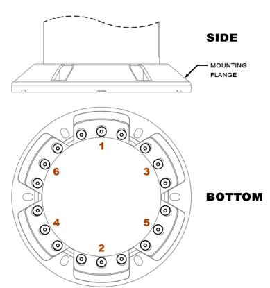
The **mounting flange** of your shock mitigating pedestal is shipped installed in the lowest position available. This torque procedure **must be followed** if loosening the fasteners to adjust the position\* of the mounting flange.
